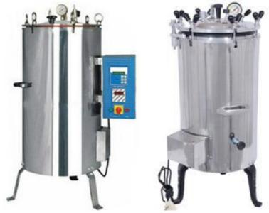
**TOPLAB INDIA'S** Vertical autoclave units are available with chamber volumes of **22 liters to 175 liters** that accommodate two and three drums accordingly. These systems are designed for meeting effective sterilization requirements in bacteriological and research laboratories, hospitals and clinics and food and beverage units. The vertical chamber design maximizes space utilization, while microprocessor control system enables comfortable working all the time you operate the machine.
